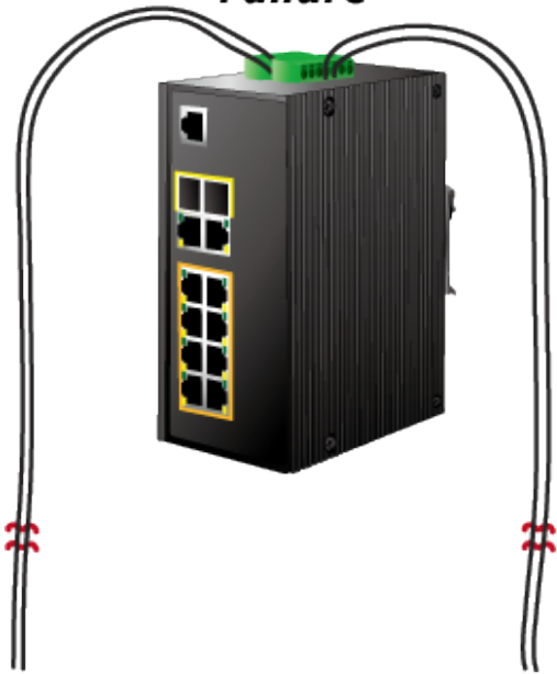
DC/DC Power Failure
